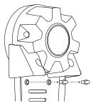
2. Pull out the stand in the direction indicated by the arrow until it is fully extended.
